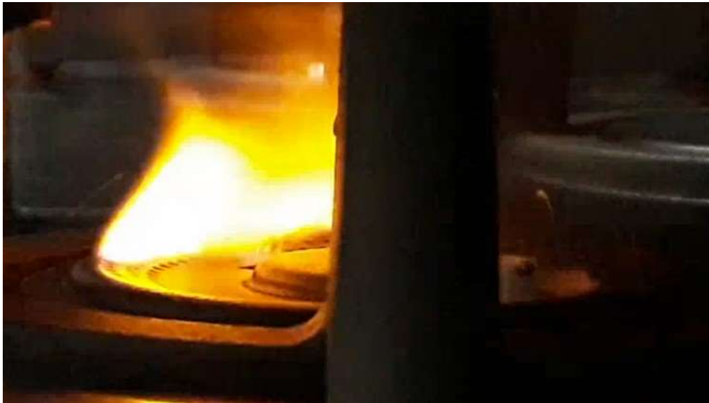
Figure 57: EN12 Burner operation when water is falling on it.
