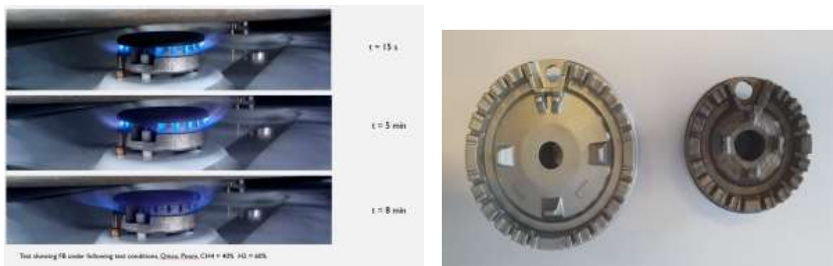
Figure 11: Impact of time on the flame (left picture) and impact of flashback on gas burners (right picture)
