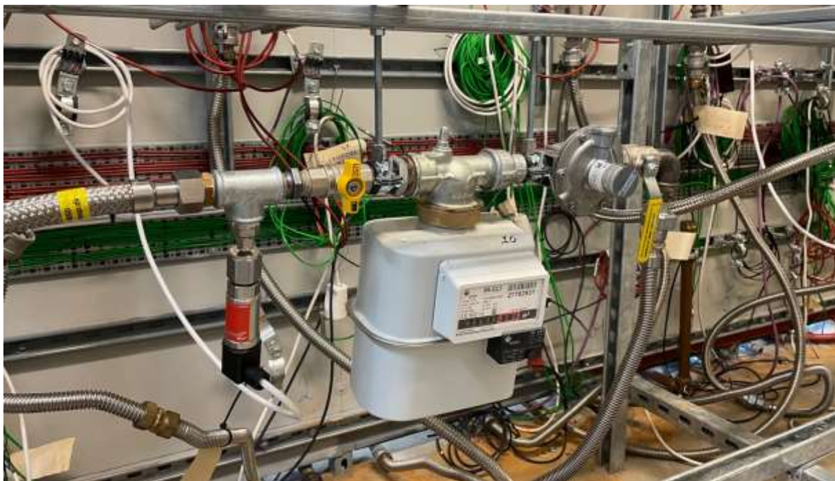
Figure 8: Instruments for the measure of the appliances (here a gas meter for boiler 1)
