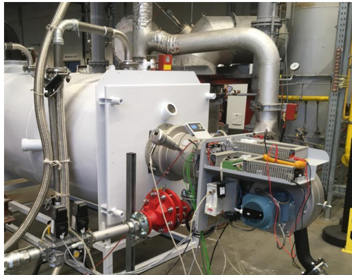
Figure 2-7 Industrial forced-draught burner installed at a burner test rig in the GWI laboratory [Hube00].
